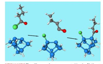
MECHANISM The silicon surface, represented by the Si<sub>9</sub>H<sub>12</sub> cluster, abstracts chlorine from butanoyl chloride and then chemisorbs the butanoyl radical. Blue atoms represent silicon; green, chlorine; red, oxygen; white, hydrogen; and gray, carbon.
