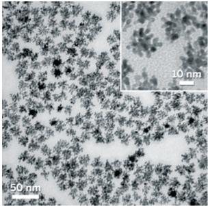
Science © 2009 Nanodendrites with Pd cores and Pt branches are highly active fuel-cell catalysts.
