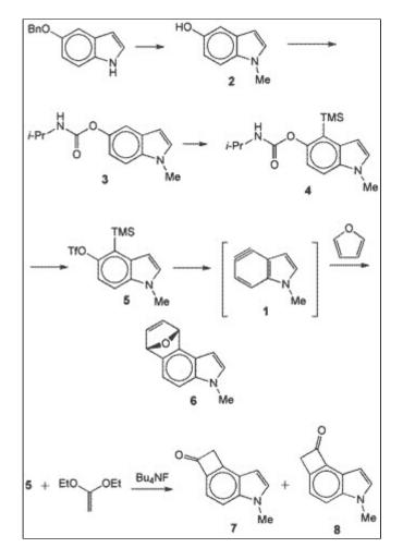
Their target structure was 4,5-indolyne (1), which is generated from precursor 5. The preparative sequence starts with commercially available 5-benzyloxyindole.
